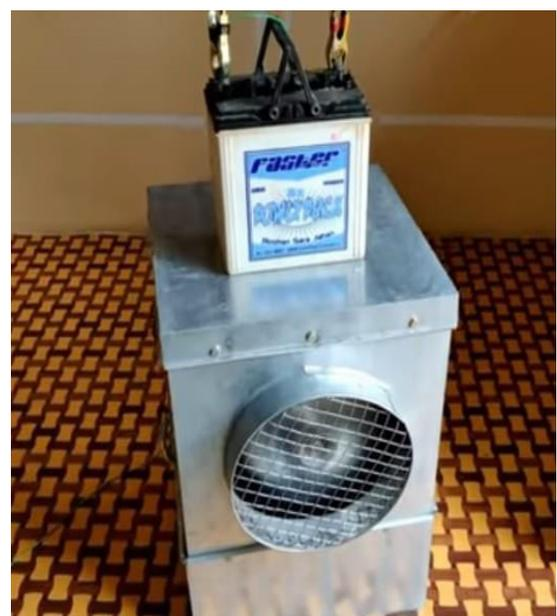
As motor start rotating the fan also start rotating. Which supply the flow of air. To cool the flow of air we use cooling system. In the Cooling system we use water as coolant.
